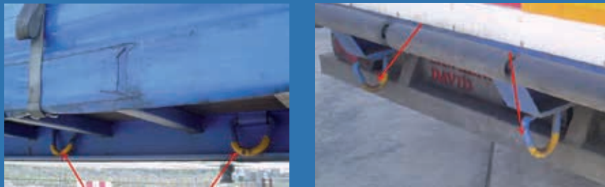
Fig no. 13 & 14 Clearly marked and well-located securing/lashing points
