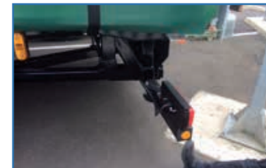
Fig no. 3 Low tail bar on semi-trailer suitable for Fork Lift 'Piggy Back'
