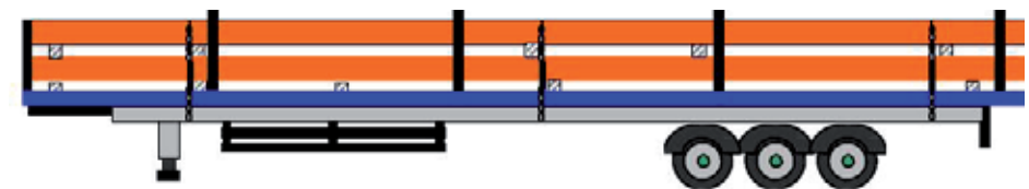
Fig no. 17 Vehicles carrying RSJ's or steel beams on a posted semi-trailer
