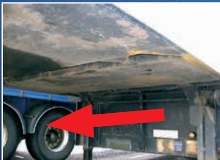
Fig no. 7 Load bearing area suitable for placement of a trestle along the marked arrows.
