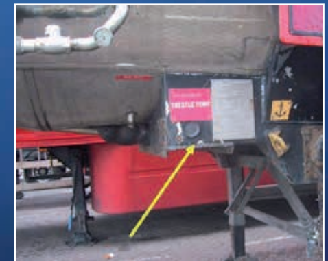
Fig no. 11 Example of a suitable trestle points on a tank unit.
